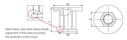
Closed end versions and different diameters (M 4 to M 12) are available on request:
